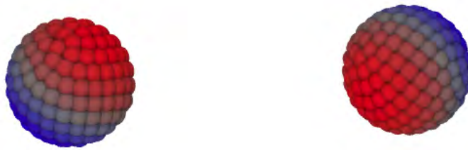
Figure 2.1. Representation of the surface function \rho(S) for two interacting particles of arbitrary orientations, where blue indicates \rho = 0 and red indicates \rho = 1 .
